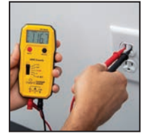
Measure Voltage at Outlets
