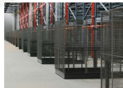
10 TRUCK AISLES The Partitioning System allows warehouse trucks to come through without compromising the safety of personnel or goods.
