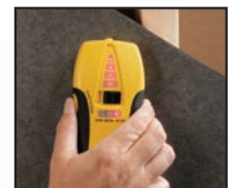
Scan for Studs, Metal and AC Voltage
