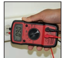
Test lead holders for one-handed testing
