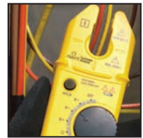
13mm Open jaw design for ease of measurement
