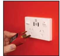
Tests outlets protected by GFCI RCD
