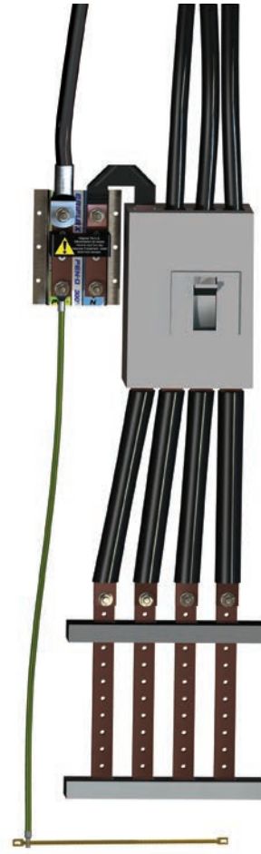
Dedicated TN-S Power Supply
