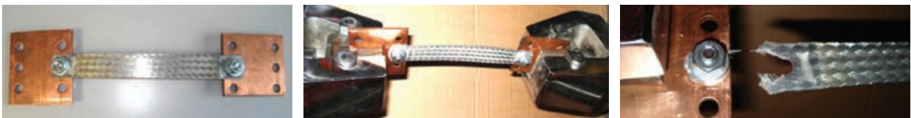
Tensile strength test sequence pictures
